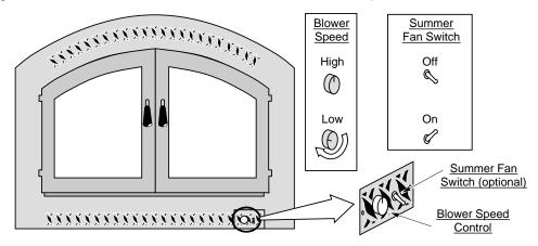
**Note:** The blower will shut off when the doors are opened.
